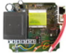
NDA008 K65 module for D-Pro Automatic control unit, for remote control (combined with NDA0006 module).
