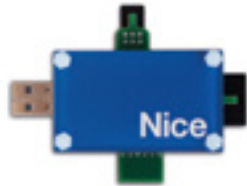
NDA004 Bluetooth module for D-Pro Automatic control unit management via smartphone.
