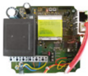
NDA008 Repeater module with integrated router.
