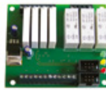
NDA030 K30 expansion module for D-Pro Automatic to add further inputs, outputs and to control traffic lights.
