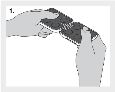
Code exchange between a memorized transmitter and a new one, to be memorized.
