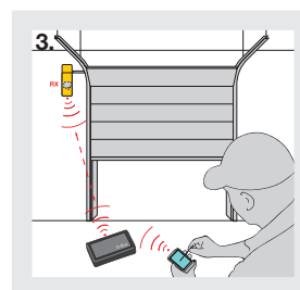
The presence of a "transmitter" in the OXIT, OX2T and OX4T receivers allows radio codes to be accessed by means of the O-Box multifunction interface.
