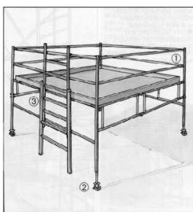
Use the scaffold means while working at height (constructional shelving with enclosures protecting from falling). These means have to be inspected and tested; they have to satisfy the EU requirements, and be certified;
